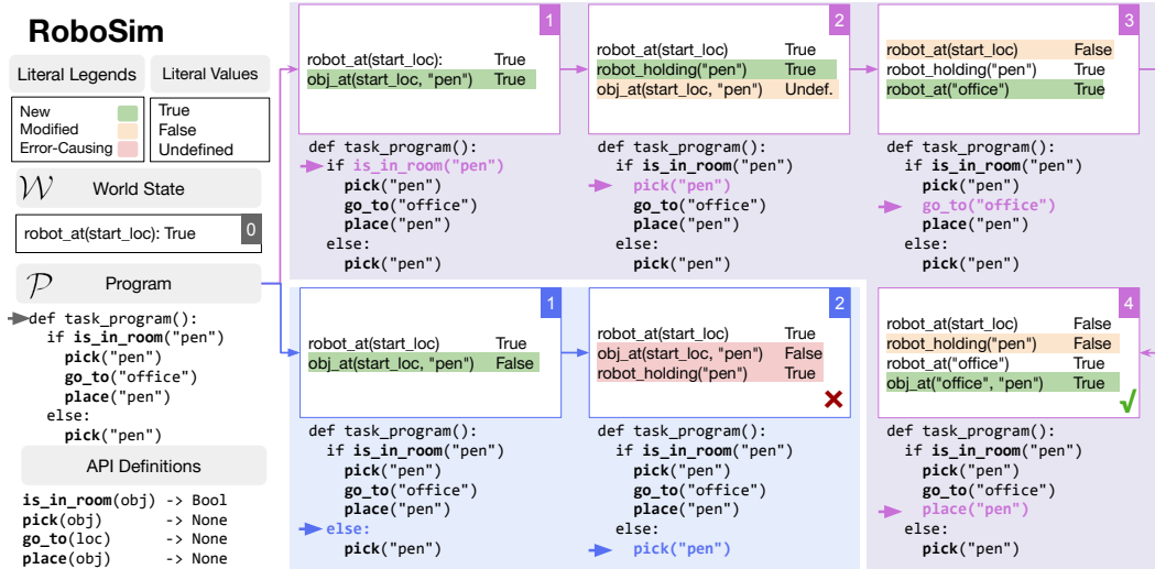
Figure 2: Example of ROBOSIM executing a generated program and updating the world state. Initially, ROBOSIM begins with a world state that includes only the robot’s current location. As the program executes, two distinct execution paths emerge, depicted in light purple and blue. This figure demonstrates how the world state is updated along each execution path.
