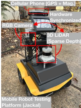
Fig. 6: Mobile robot testing platform for real-world experiments. We annotate the locations of the monocular camera, 3D LiDAR, and cellular phone (not visible) on our testing platform, the Clearpath Jackal.
